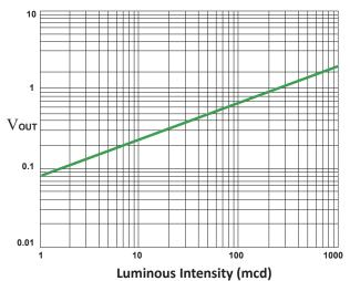
Typical response for PLCC green LED tested with Universal LightProbe Penta Sensor and Small-Aperture Fiber-Optic Probe
